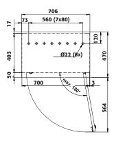
Diagram shows left-hinged door. Dimensions are identical for a right-hinged fitting.
